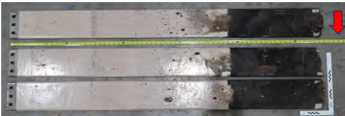
Fig. 87. Photo of Experiment 2-41 bus bars post-experiment (arc location at arrow).
