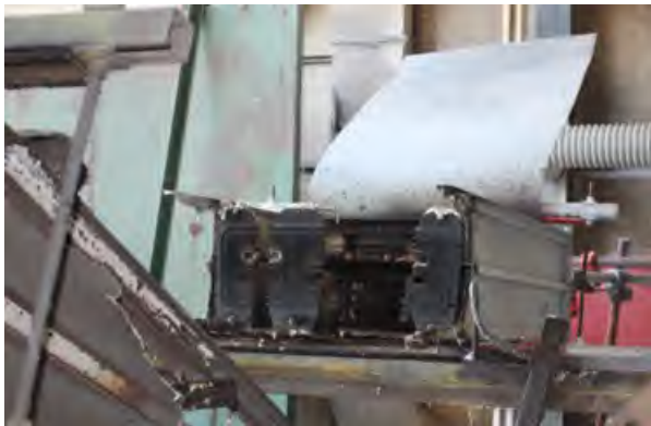
Fig. 203. Post-Experiment 2-40 Bus Duct. Left – horizontal duct with copper bars at support, Right – end of severed duct as viewed from incoming power side.
