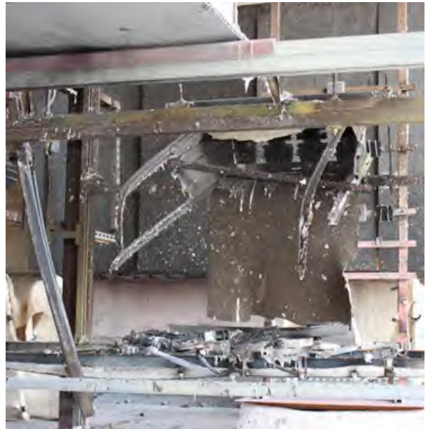
Fig. 203. Post-Experiment 2-40 Bus Duct. Left – horizontal duct with copper bars at support, Right – end of severed duct as viewed from incoming power side.
