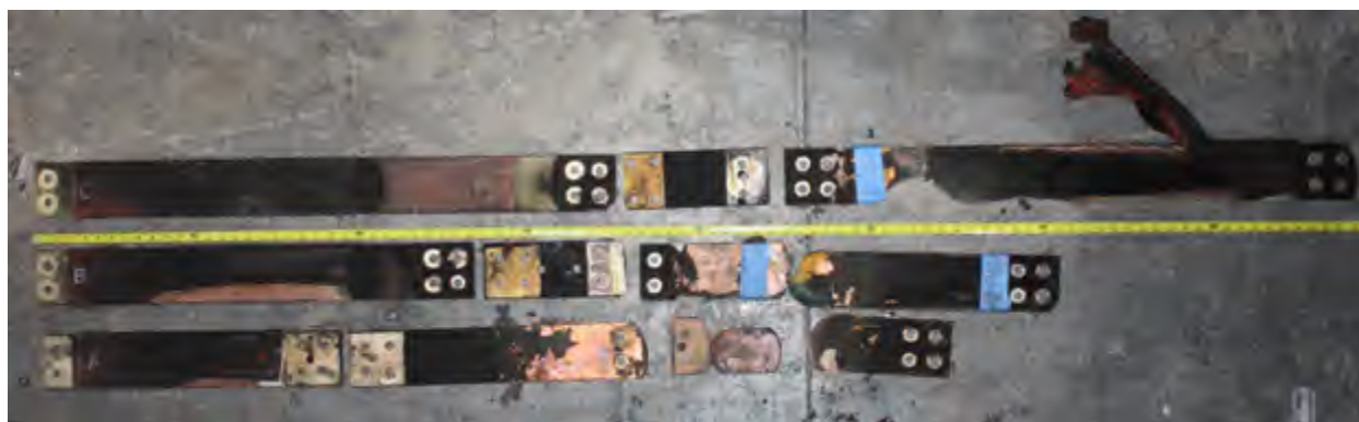
Fig. 64. Photo of Experiment 2-37 bus bars post-experiment.
