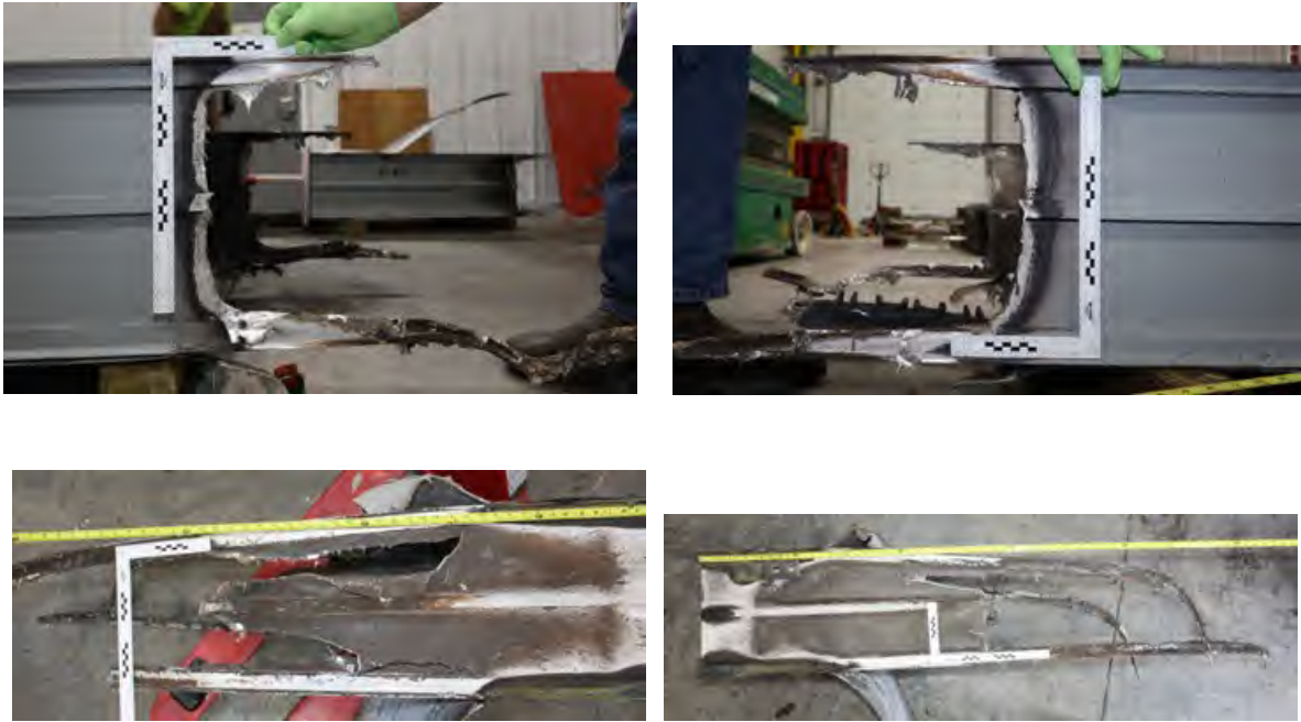
Fig. 204. Post-Experiment 2-40 Duct Enclosure Breach.
