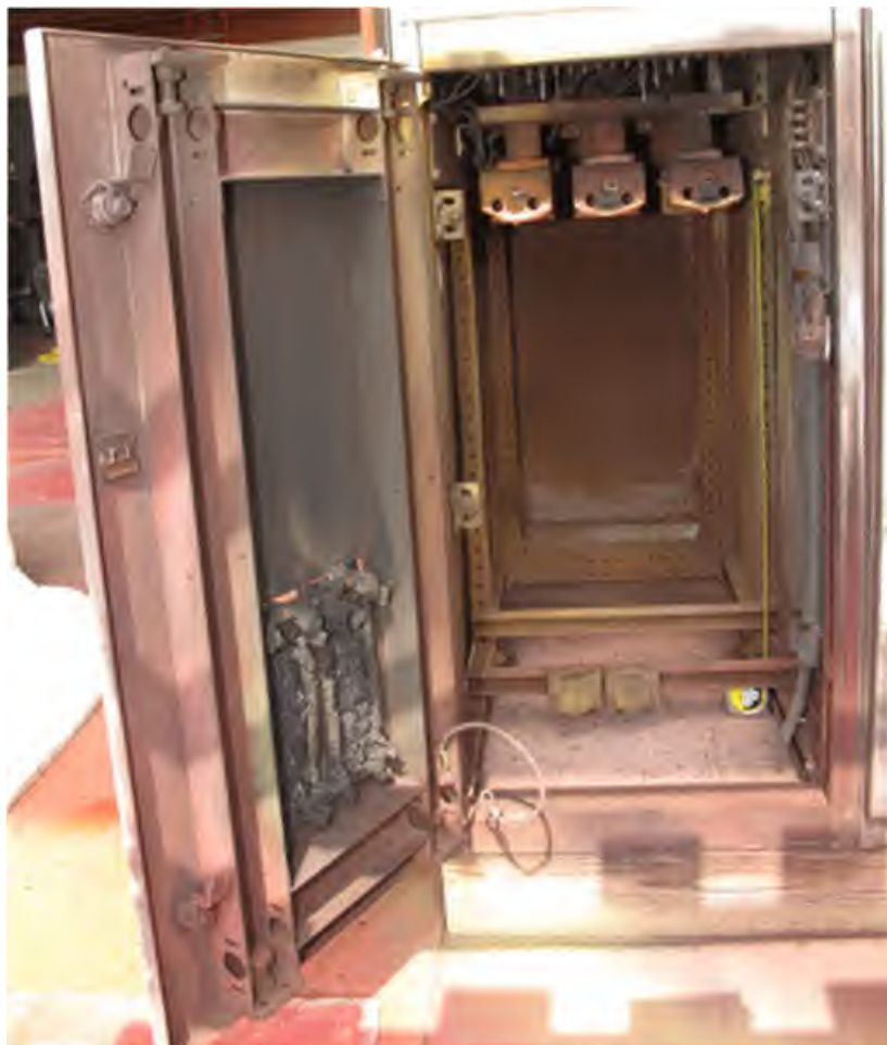
Fig. 163. Post-Experiment 2-33A Conductors. Enclosure 'C' (EV53).
