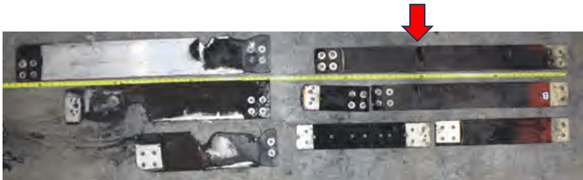
Fig. 70. Photo of Experiment 2-38 bus bars post-experiment (initial arc location shown by arrow).
