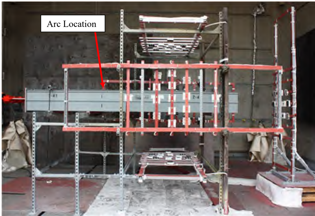
Fig. 205. Pre-Experiment 2-41 Bus Duct. Duct and instrument rack configuration prior to experiment.
