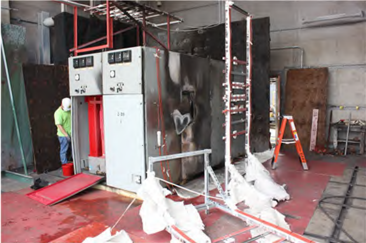
Fig. 197. Post-Experiment 2-39 Enclosures “M”, “I”, and “K”. Note door to Enclosure “M” is not in photo, instrument rack positioned in front of Enclosure “I” fell to the ground after impact from Enclosure “M” door.
