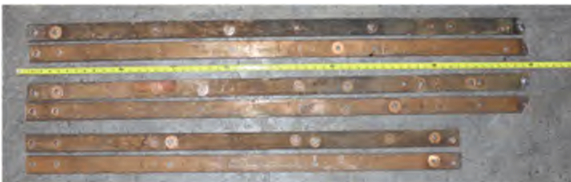
Fig. 44. Photo of Experiment 2-34 bus bars post-experiment (arc location shown right).
