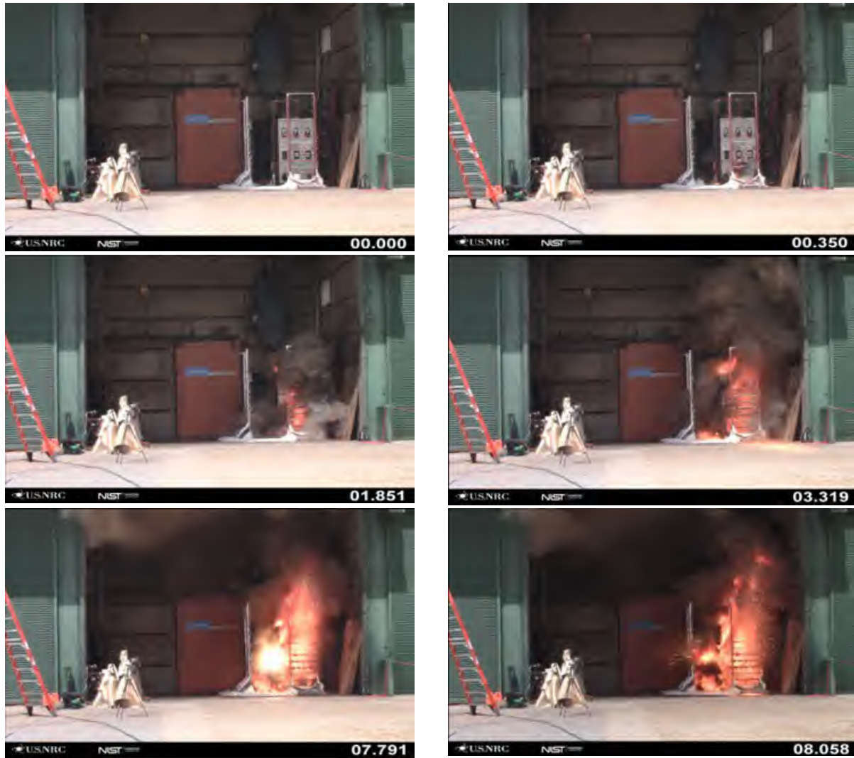
Fig. 35. Sequence of Images from Experiment 2-33B (image time stamps are in seconds).
