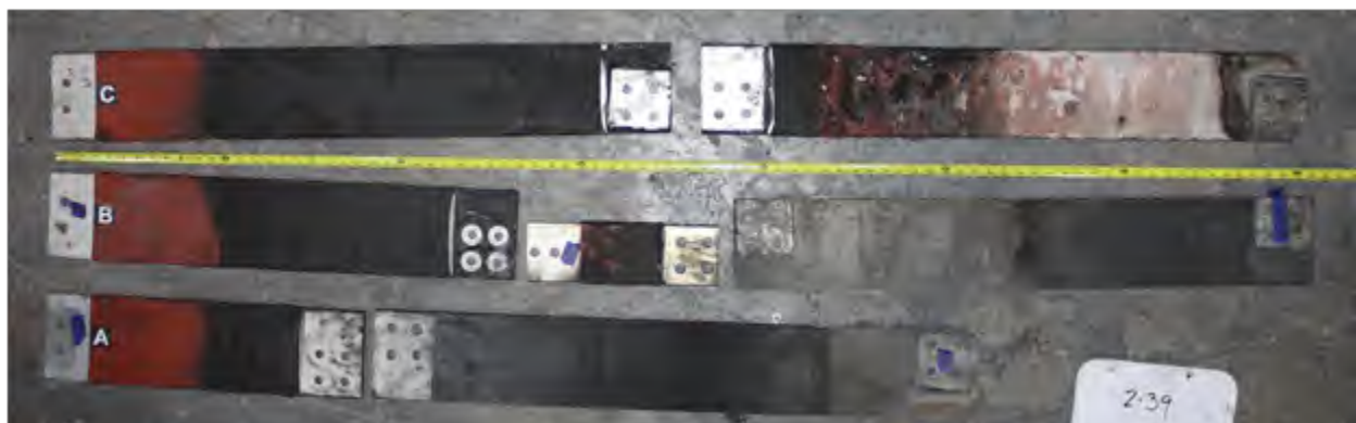
Fig. 76. Photo of Experiment 2-39 bus bars post-experiment.
