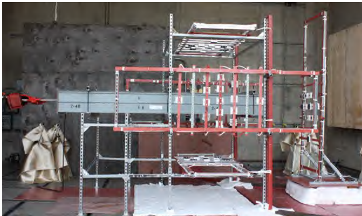
Fig. 28. Photo of bus duct instrumentation configuration prior to experiment
