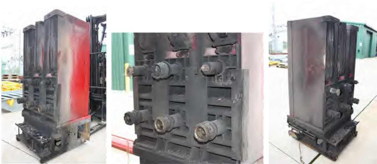
Fig. 187. Post-Experiment 2-37 Breaker. Left - rear angle view, Center – stab close-up, Right - rear angle view.
