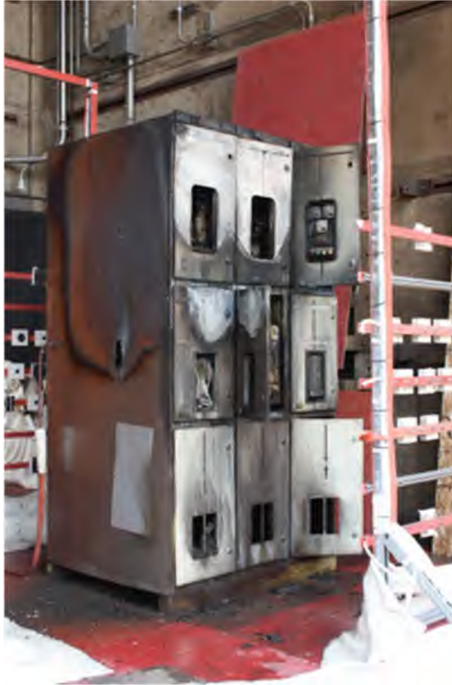
Fig. 37. Enclosures Post-Experiment 2-33B. Note the external breach on the middle side panel of Enclosure ‘C’.
