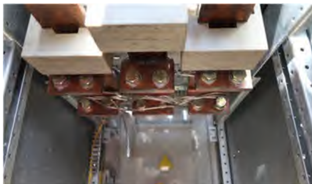
Fig. 213. Pre-Experiment 2-XXA. Arcing wire location.
