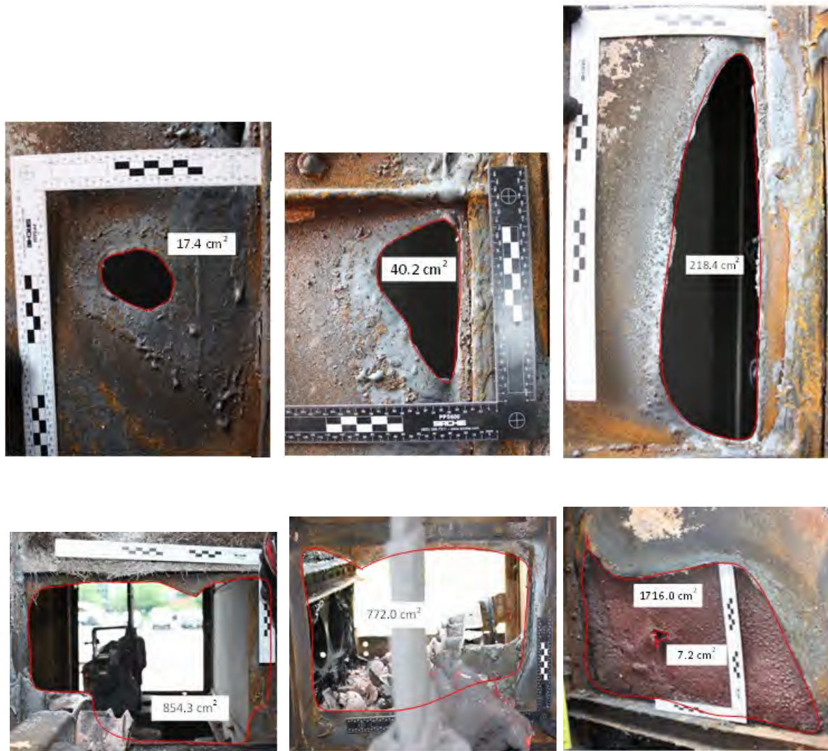
Fig. 185. Post-Experiment 2-36, Enclosure "H" breaches.
