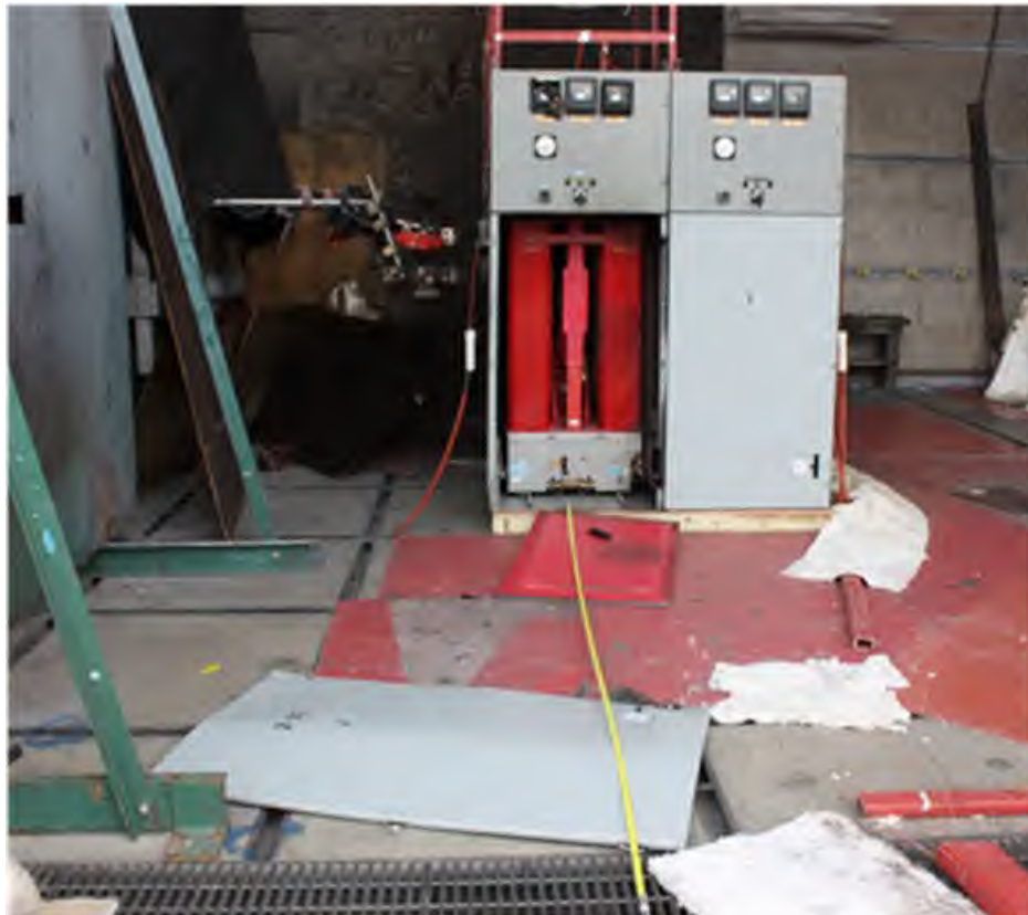
Fig. 60. Post-Experiment photo of Experiment 2-37 showing resting place of Enclosure “J” front door and breaker front cover.
